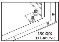
Anchor the First Level Module Plates Figure 21-8
