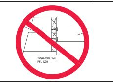
Anchoring to a wooden floor (not recommended) Figure 22-10
