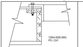
Anchoring to a wooden floor (preferred method) Figure 22-9
