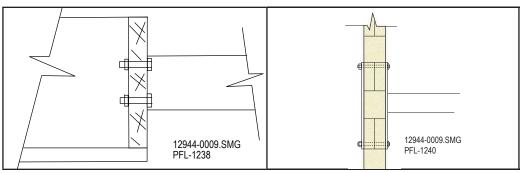
Anchoring to a wood floor - through bolting Figure 22-7
