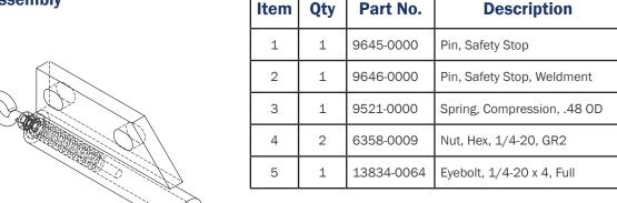
Prior to assembly apply Loctite® #242® Blue Threadlocker to internal threads only. Keep exterior of pin clean.
