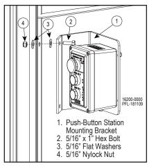
Attach Push-Button Station Mounting Bracket Figure 23-1
