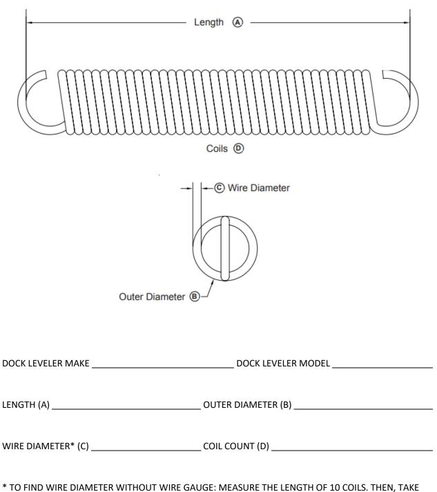
THE MEASUREMENT AND DIVIDE BY 10 TO DETERMINE WIRE SIZE.
