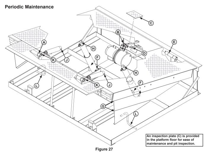
A-Lip Hinge Area D- Dual-Lanyard Lever Pivot B- Logic Block Valve Lever Pivot E- Platform Hinge Area **C**— Inspection Plate F— Frame Cylinder Trunnions
