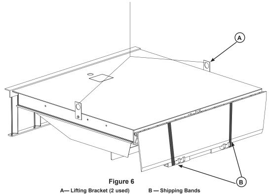
Poweramp dock levelers are shipped with lifting brackets (**A**) fastened to the platform side joists, and shipping bands (**B**) around the platform lip and leveler frame (see Figure 6).
