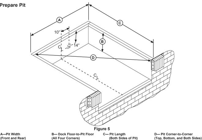
Before lowering the dock leveler into the pit, the following must be performed:
