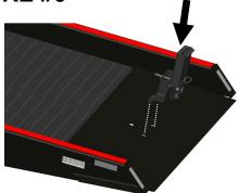
1. Stand the positioning sleeve vertical and insert the positioning sleeve lugs into the rectangular cutouts in the approach plate of the ramp.
