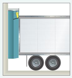
The exclusive pivoting head member of the WeatherGuard unit automatically adjusts to the height of the vehicle when positioned at the dock.
