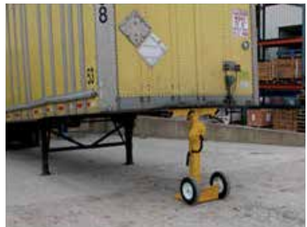
Heavy duty trailer stabilizer shown under trailer
